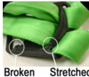
Figure 10: Visual signs of harness damage
